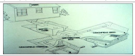
When a Septic System is working properly, wastewater leaves the building through a main pipe and enters the Septic Tank. Here, the solids separate from the wastewater and naturally occurring bacteria work to biologically break solids down. Fluids move on to the distribution box and are distributed to the Leachfield area. These fluids then drain downward into the soil. Pollutants are treated in the soil as cleaner water continues downward.
