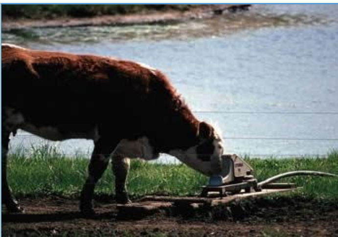
Photo courtesy of USDA NRCS. Nose-operated demand pump draws water from nearby surface water and eliminates shoreline access.
