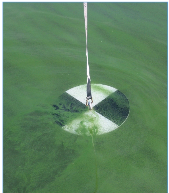
Above: A secchi disc is used to measure turbidity in a waterbody undergoing an algae bloom.
